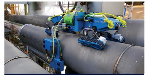
Scanning a full pipeline diameter using the multi-view approach of the 2-axis arm
